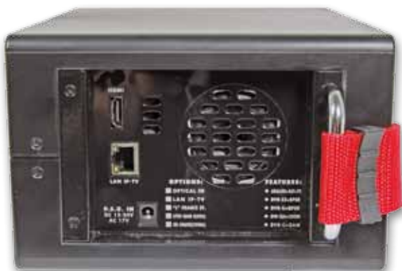
The left side panel has an HDMI output to connect an external HD TV or monitor, the LAN IPTV socket for IP television channel tests, structured cabling and the 12V power supply socket.
