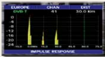
ECHO MEASUREMENT, impulse response, the only one in real time to minimize Digital Terrestrial interferences.
