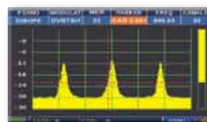
MER Versus CARRIER measurement for carriers (optional)
