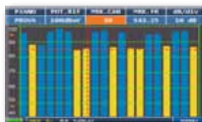
Bars Scan TV & CATV function from 10 to 100 channels ▬ analog ▬ digital
