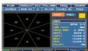
DVB-S2 multistream Constellation 8PSK mod., on the right relative modulation parameters & ISSY
