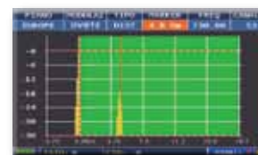
MICROECHO MEASUREMENT in SFN networks, with impulse response in real time and relative guard interval
