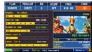
All the measurements, A/V PID, the picture and settings on one screen
