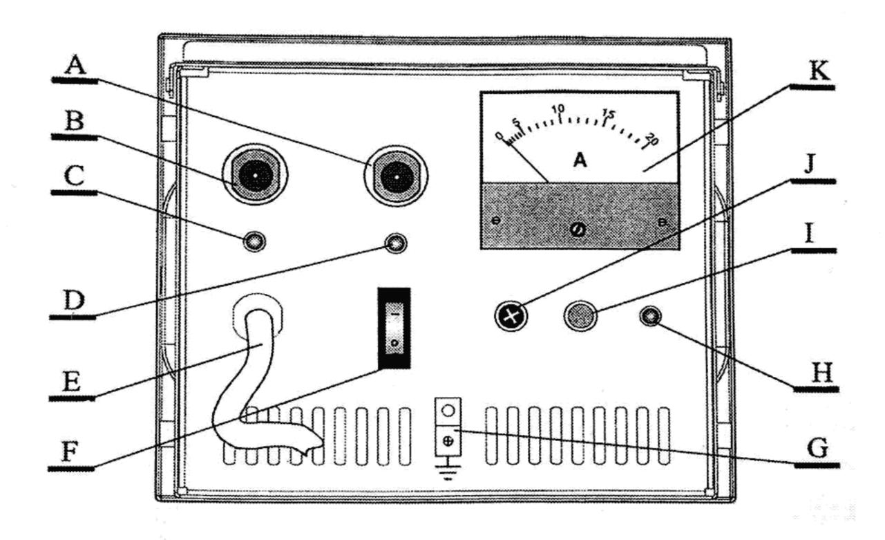
A.60V output II: AC60V/RF signal output port.
