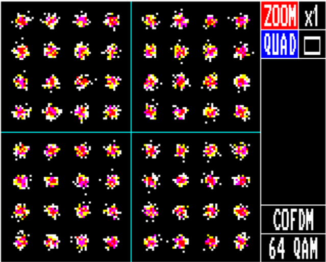
COFDM-64 QAM constellation example
