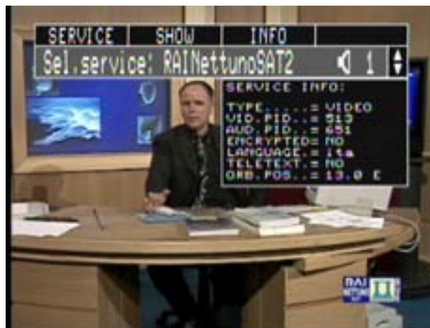
Example of a picture and relative data from the indicated transponder, obtained using the "SERVICES" selection contained in the menu associated with digital signals.
