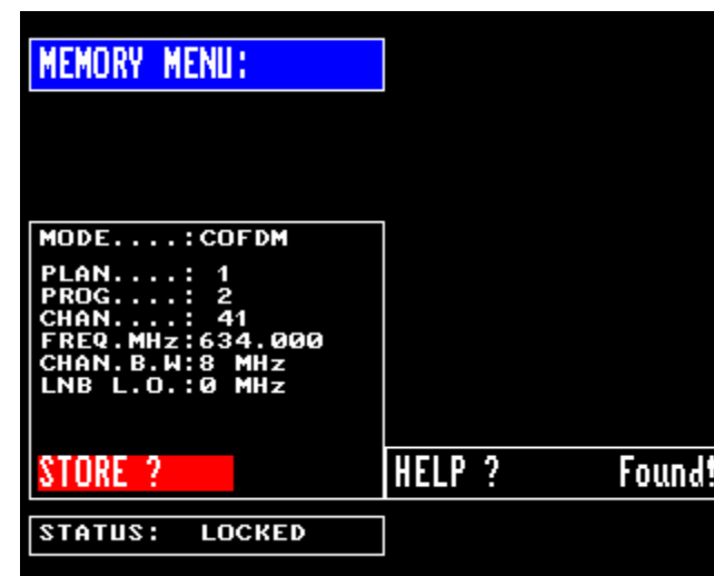
Once the search has finished, the cursor moves to STORE? or OVERWRITE? press ENTER per save.
