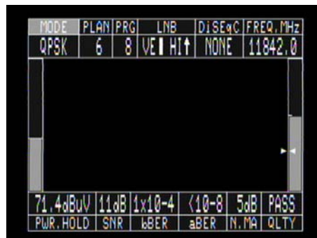
Fig.7 QPSK measurement, level 2, with power bar to the left and quality to the right, the white arrow shows the suggested minimum quality.
