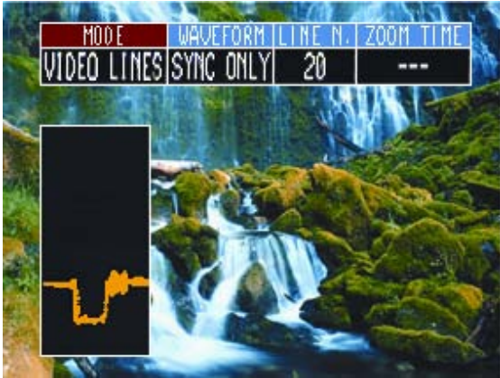
SYNC ONLY Synch. pulse visualisation
